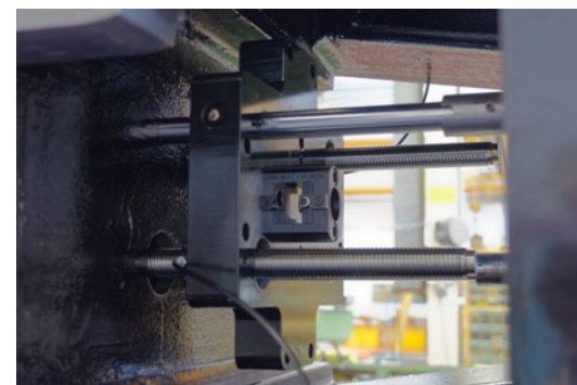
⌚ VERSATILE CROSS PLATE EJECTION SYSTEM
